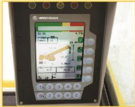
力矩限制器采用彩色液晶显示器，实现故障诊断智能化，精度领先于同行业。 Load moment limiter with color LCD realizes intelligent trouble diagnostic, and its precision leads in the same-class products in the industry.
