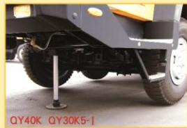
扩展了起重作业的空间可范围，极大提升了前方区的起重能力。 Expanded lifting space and range increase greatly the lifting capacity over front.
